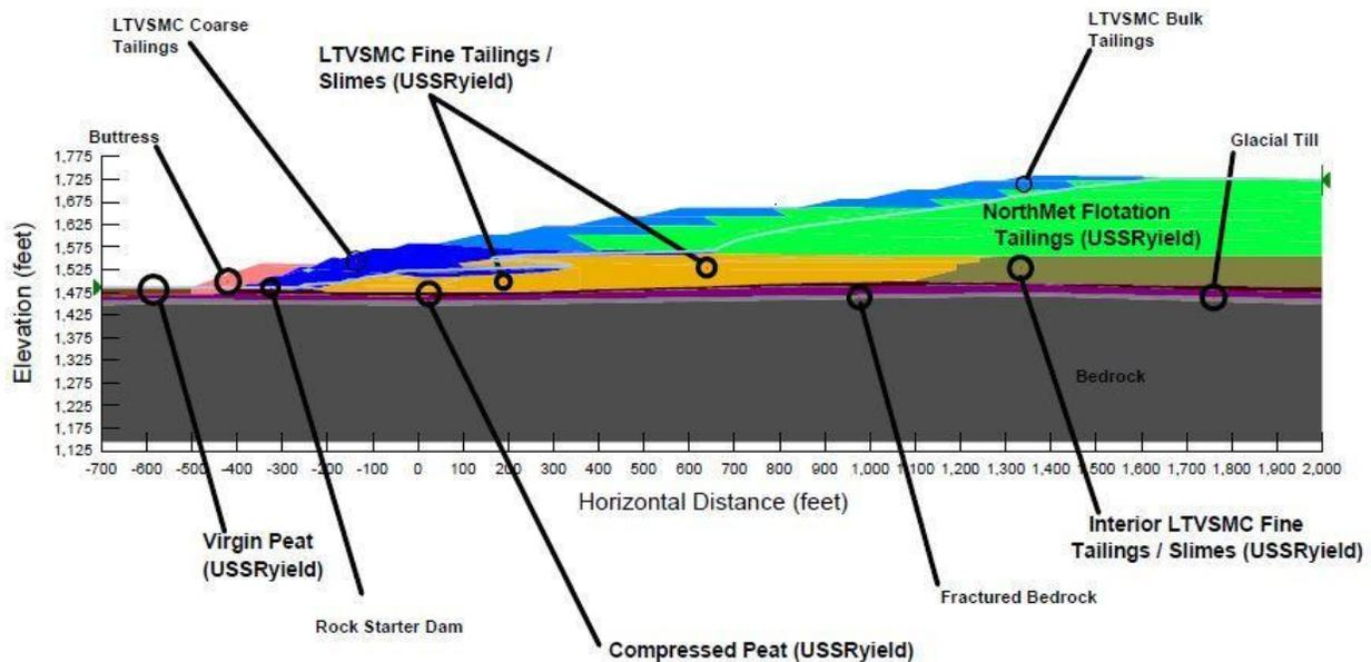
**Large Figure 12. Cross-Section F Schematic of USSA Conditions**
